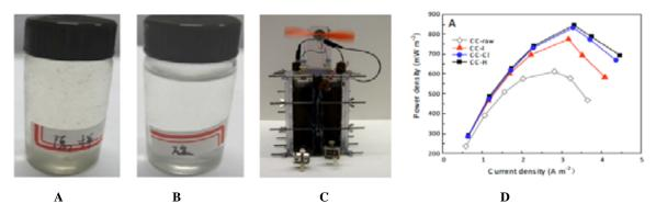
Fig. (1). Bioelectrochemical system for Wastewater treatment: (A) before treatment; (B) after treatment; (C) power from wastewater to drive a fan; (D) Power density for MFCs with the raw and treated anodes.
